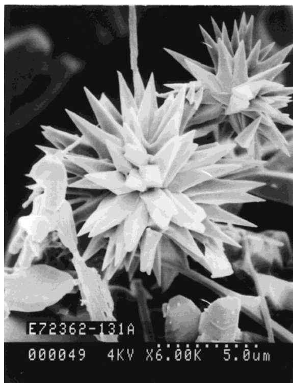
Figure 5. Scanning electron microscopy revealing the particle morphology of COET mixture prepared in hexadecane and crystallized by slow cooling to room temperature. These morphologies melt at ca. 304 °C.
